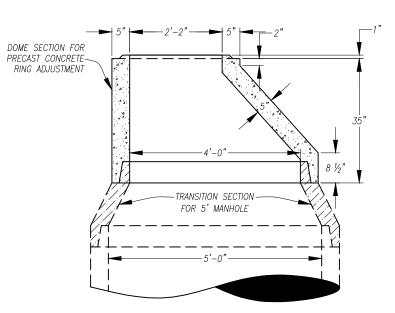
4'-0" FOR SEWERS 24" AND UNDER, STD. MANHOLE No. 3 5'-0" FOR SEWERS 27" TO 42", STD. MANHOLE No. 4
